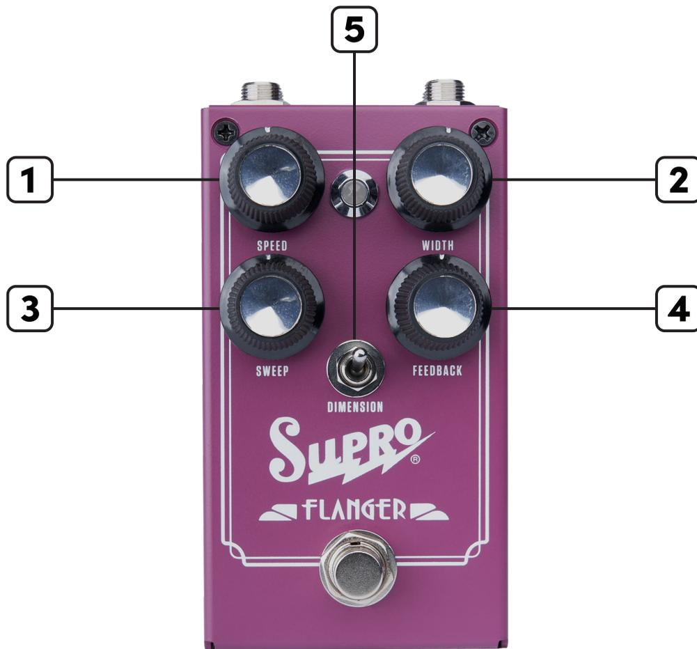
**1** **Speed:** Sets the rate of modulation of the Flanger effect.
